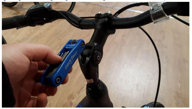
BEFORE tightening the nut, you may set the height of the handlebar, but be aware that there is a maximal height marked on the stem, that you shouldn't exceed.
